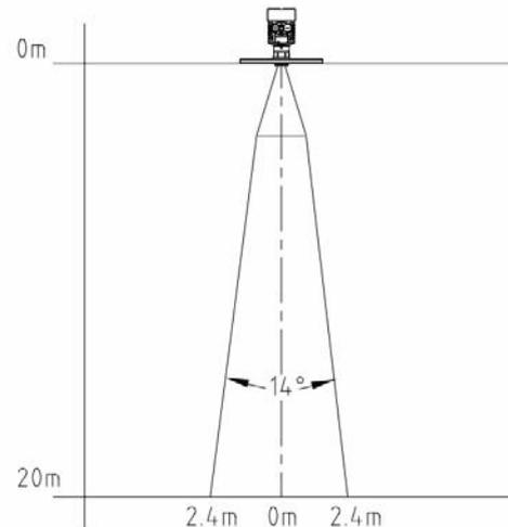
DN250 Horn antenna beam angle
