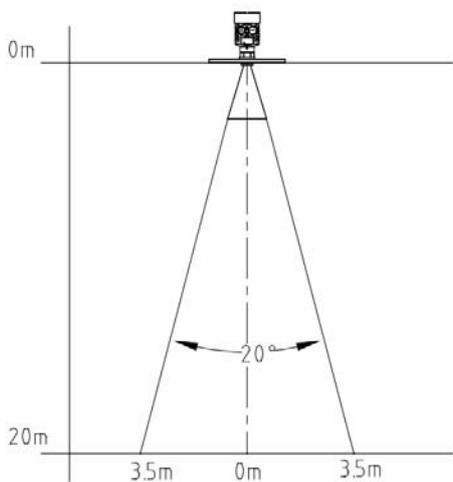
DN150 Horn antenna beam angle
