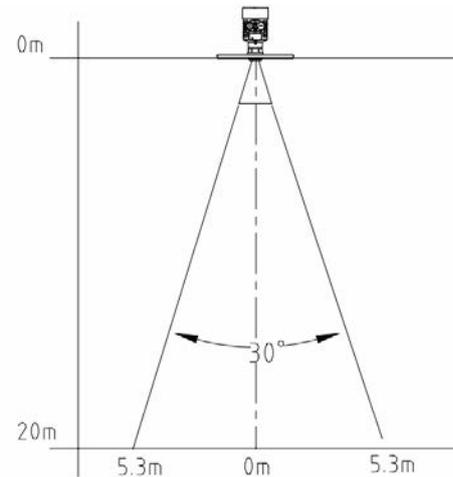
DN100 Horn antenna beam angle
